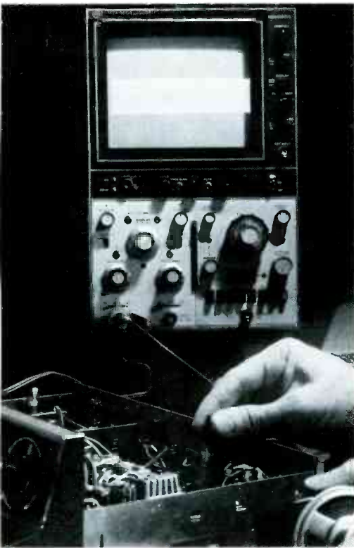
Fig. 5 Key the microphone with the same hand that holds the 1000-Hz signal-injection speaker. You can tune coils with your other hand. Modulation helps you see what's really happening to signals in the transmitter, and reveals troubles that occur.
