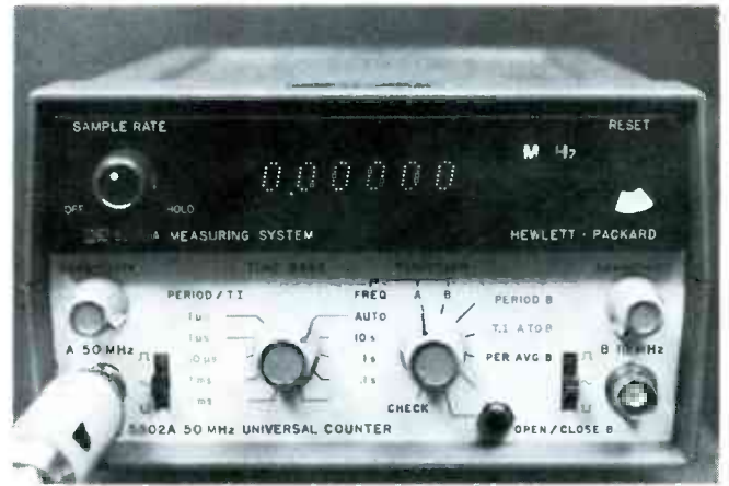
Fig. 3 Readout shows zero on the frequency counter when there's no input. Keying the transmitter, with input hooked to outer tip of 10K resistor in homemade dummy load, causes frequency to appear.
